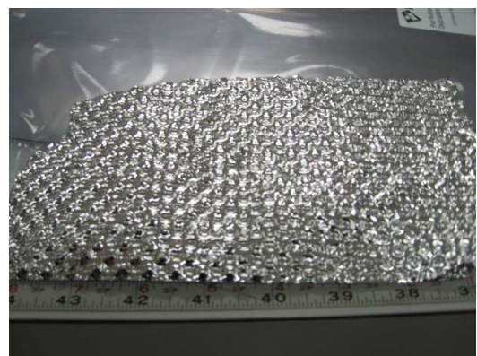
Sheltherm™ pattern has 3,850 dimples/SQ FT with a profile height of 0.060"
